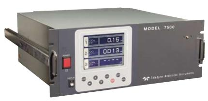
A high-sensitivity mass flow sensor is utilized for infrared measurements. By using a single beam, single path design in conjunction with a serial dual-layer transmission detector, the 7500 delivers long-term, drift-free performance. The oxygen concentration in the sample gas can be detected by either a built-in paramagnetic sensor or an externally mounted, in-situ-based zirconium oxide sensor.
