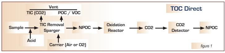
Acid is added to the sample, lowering its pH to approximately 2.0, at which point the carbonates present in the sample are converted to dissolved CO2.
