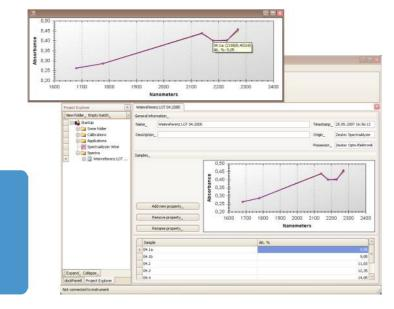
After sample acquisition, create MLR calibrations with the aid of the powerful calibration wizard. Using full combination search, it calculates every possible calibration and presents a well-chosen subset to you. The expert can browse these calibrations with an easy-to-grasp weight and score system and select the appropriate one. The layman can safely accept a calibration the wizard proposes.
