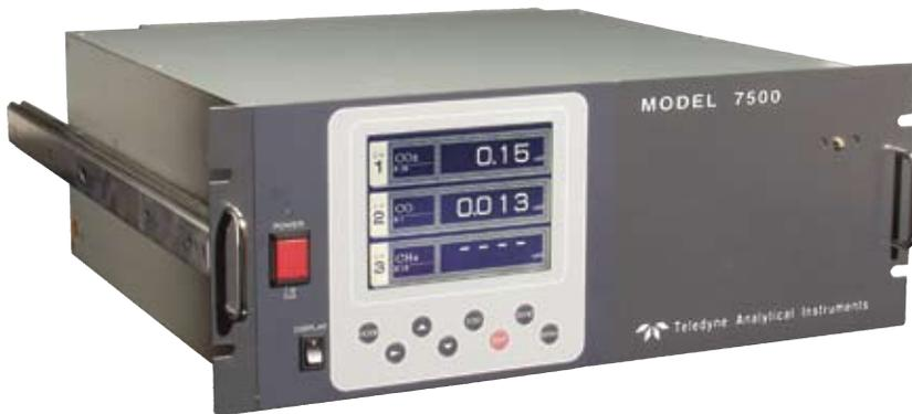
A high-sensitivity mass flow sensor is utilized for infrared measurements. By using a single beam, single path design in conjunction with a serial dual-layer transmission detector, the 7500 delivers long-term, drift-free performance. The oxygen concentration in the sample gas can be detected by either a built-in paramagnetic sensor or an externally mounted, in-situ-based zirconium oxide sensor.
